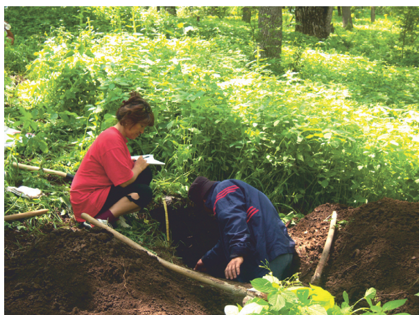
Figure 4 Preparation of a soil profile for soil layer characterization and soil sampling, nut-fruit forest, Kara-Alma, 2007
