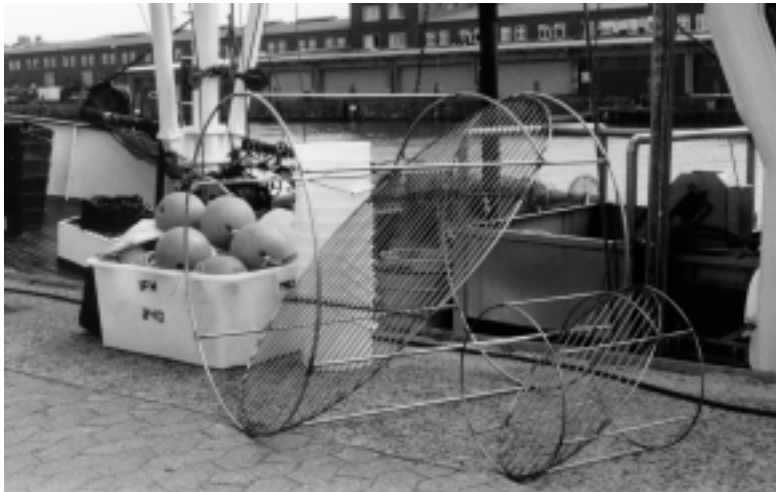
Abb. 1: Trenngitter aus Edelstahl mit 20 mm Stababstand Sorting grid made of stainless steel with 20 mm space between the bars
