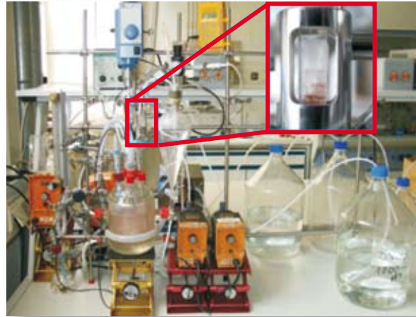
Abb. 12: Photo des kontinuierlichen Rührkesselreaktorsystems (vergrößert: Ultraschallseparator) – Photo of the continuous-flow stirred tank reactor system (ultrasonic separator enlarged)
