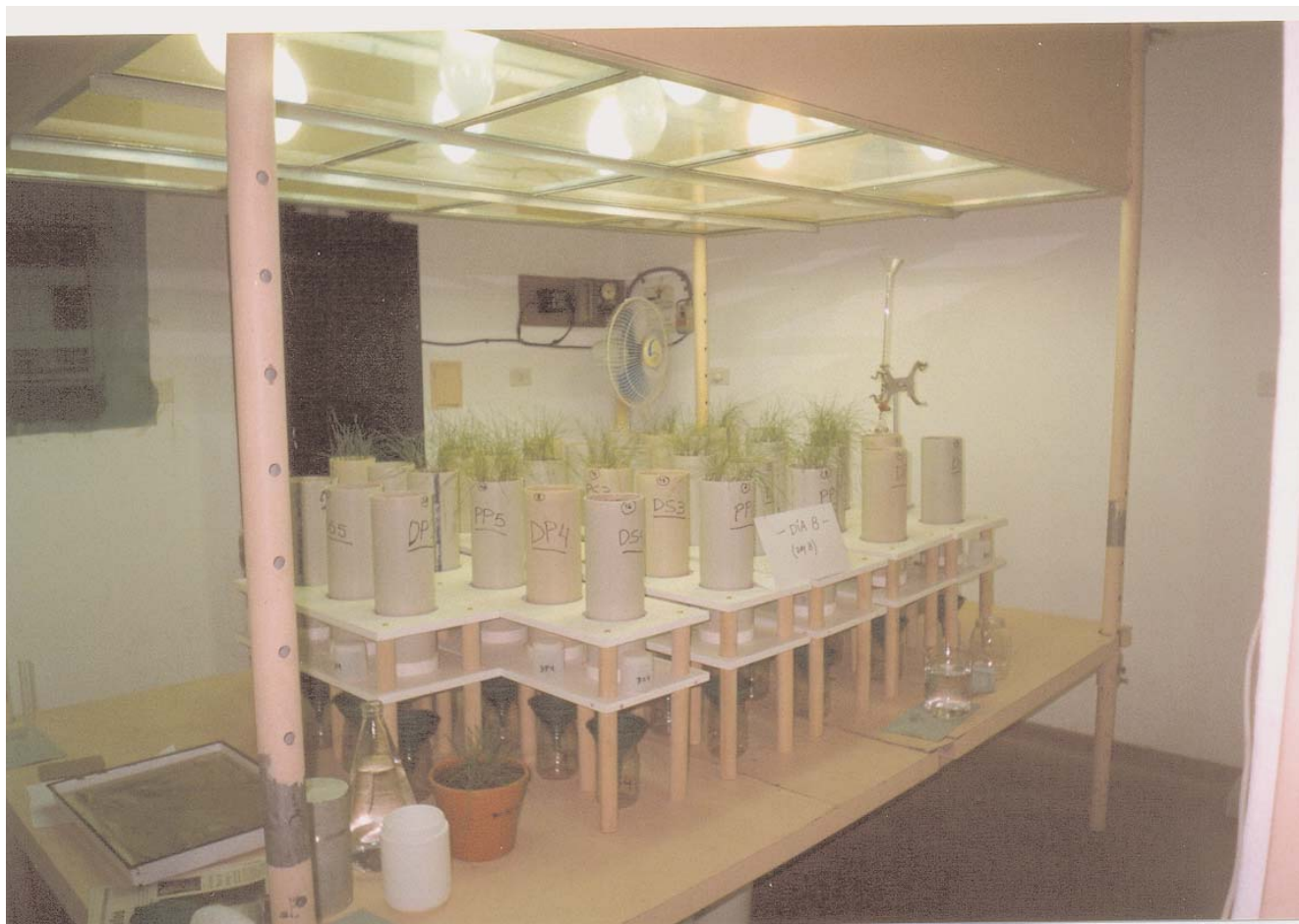
Fig. 2: View of the column experiment for the investigation of Uranium leaching during short term application of pit-water on a high-carbonate-content soil in the Mendoza province of Argentina
