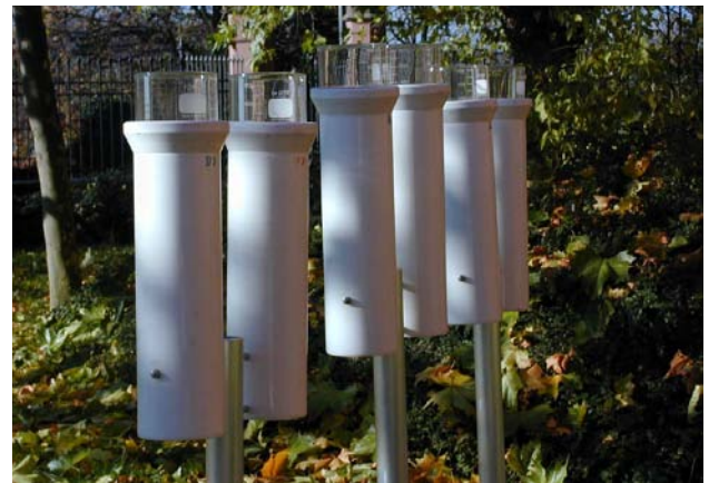
Fig. 2 Three sets of Rotenkamp samplers. Each set comprises two samplers - one sampler stabilized with hydrochloric acid and one with sodium hydroxide solution.
