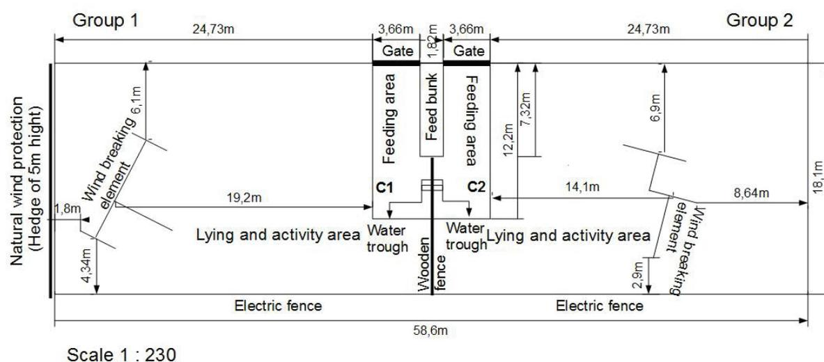
Figure 2: Layout of the experimental set-up
