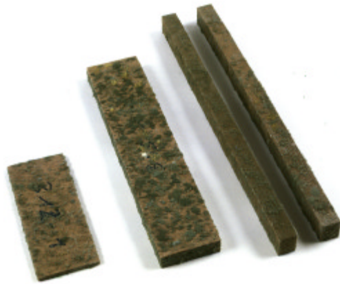
Figure 10: Nipa MDF board covered with fungi after storage in very humid climate
