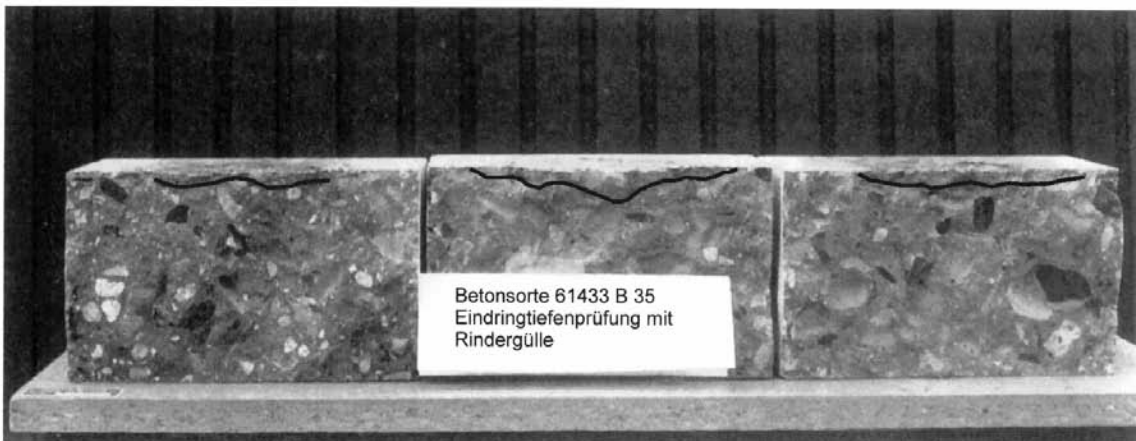
Penetration test with slurry from cattle concrete quality B 35
