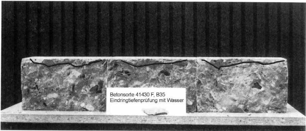
Penetration test with water concrete quality B 35
