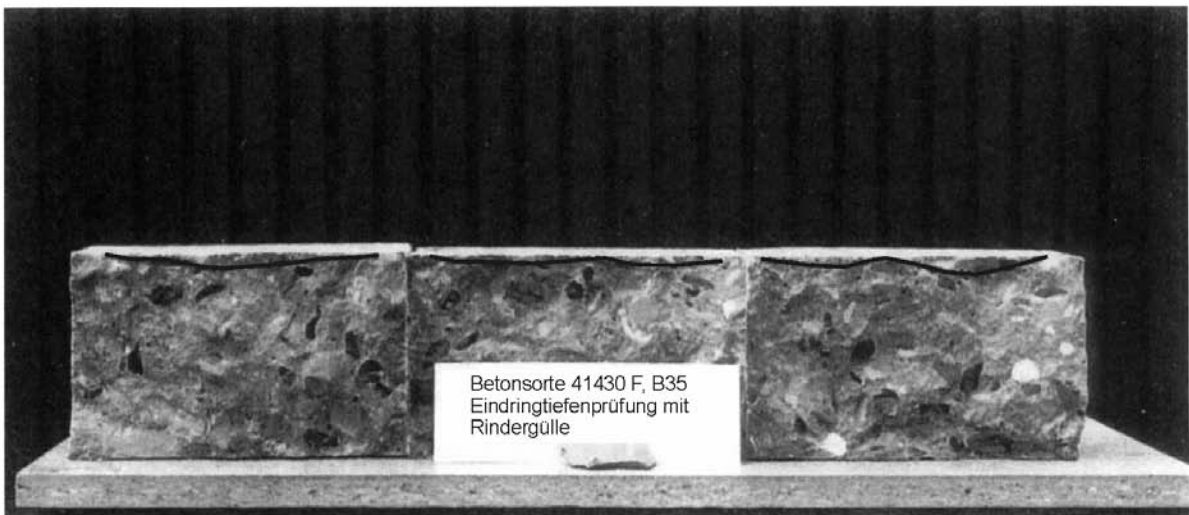
Penetration test with slurry from cattle concrete quality B 35
