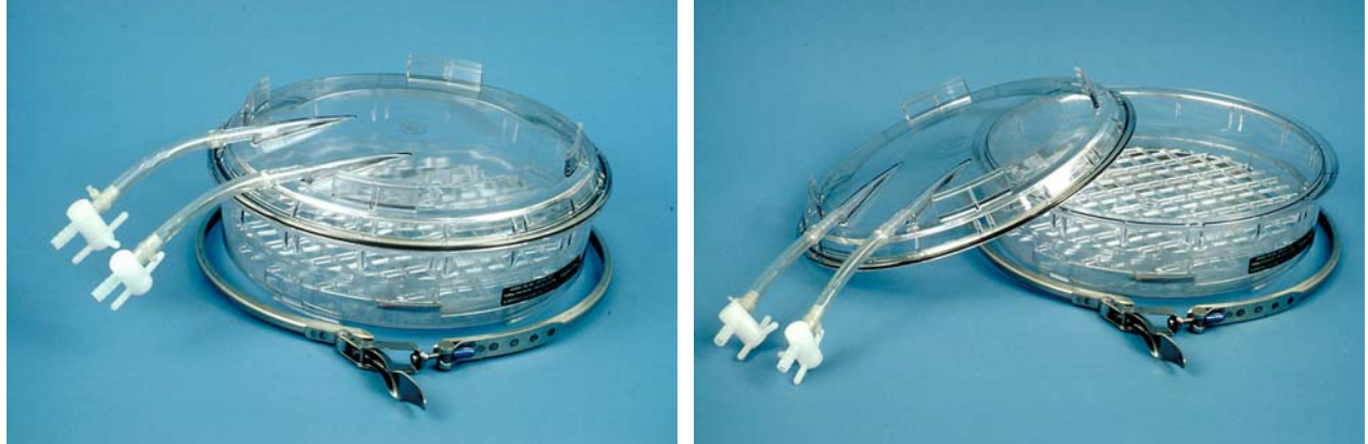
Fig. 5 Modular incubator chamber (closed and opened).
