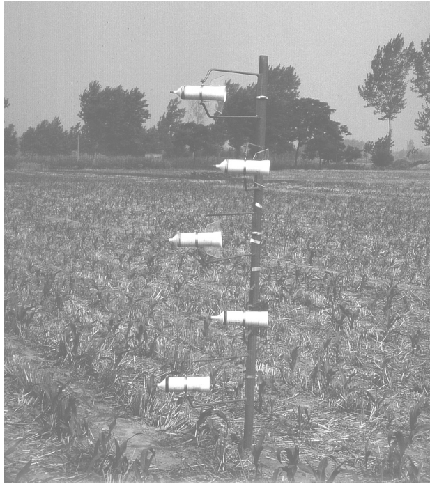
Fig. 8: Measurement pole equipped with SSM samplers (Leuning et al. 1985) in Fengqiu (maize crop)
