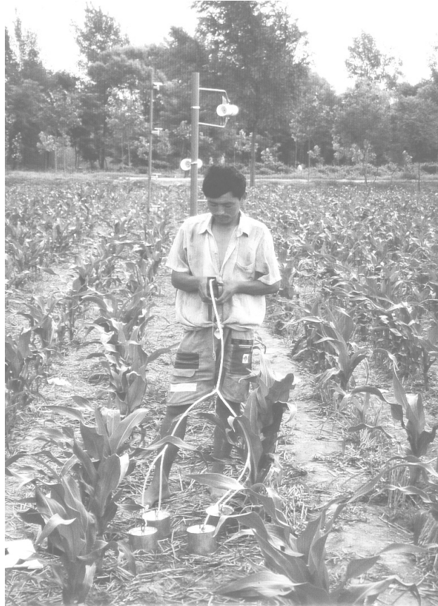
Fig. 5: Draeger-Tube measurement (hand pump) in Fengqiu; in the background: micrometeorological measurement pole
