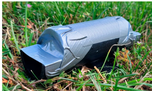
Figure 1. Hair tube for small mammals, based on the design reported in Chiron et al. (2018) [11]; © J. Dürger, JKI.
