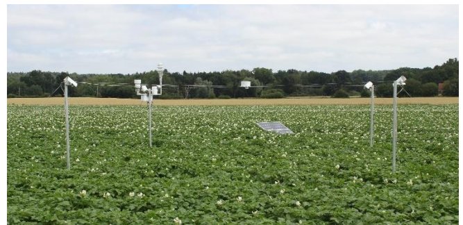
Fig. 1: Infrared temperature sensors and weather measurement equipment on a potato field, year 2018.
