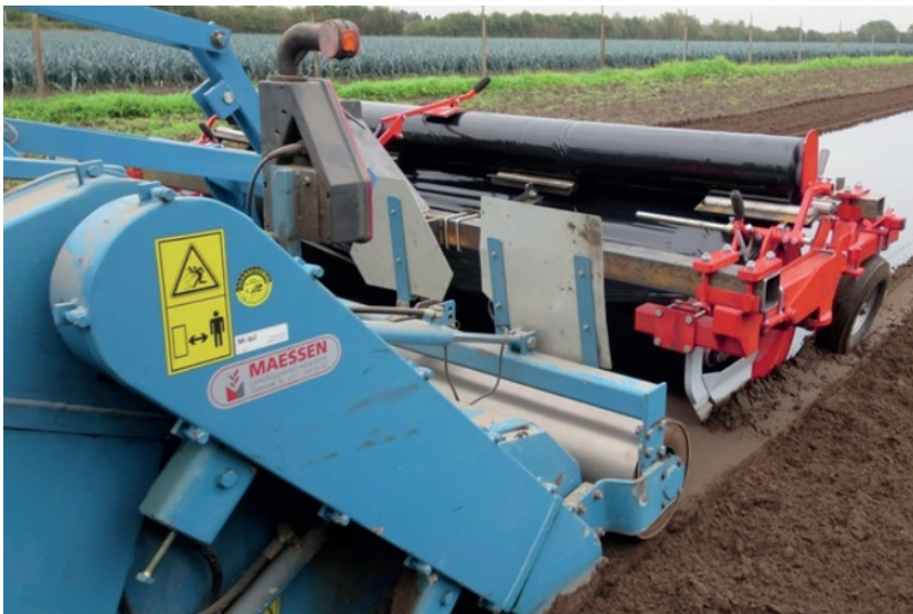
Figure 3: Injecting the disinfectant and automatic plastic covering.
