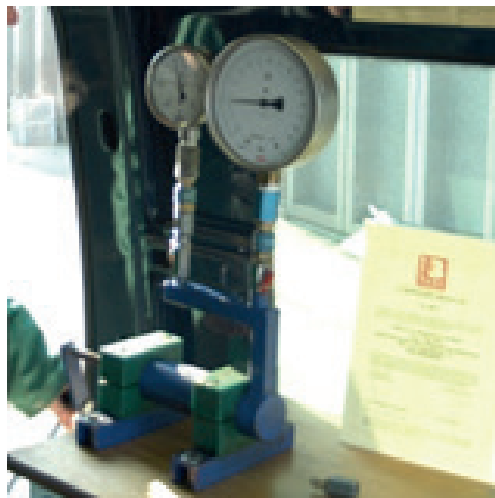
Figure 24: Pressure gauge test stand.
