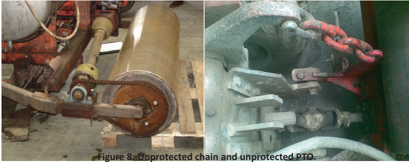
Figure 8: Unprotected chain and unprotected PTO.
