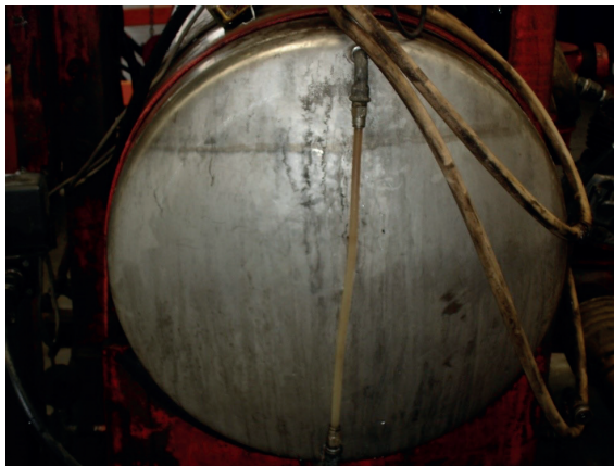
Figure 23: Tank contents indicator without measuring scale.
