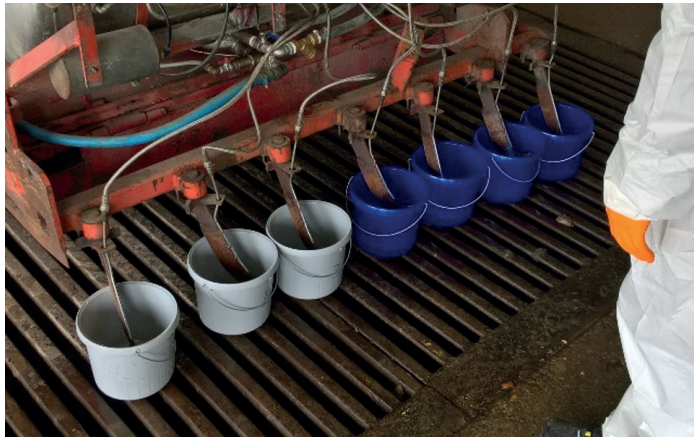
Figure 16: Pattern determination using buckets.
