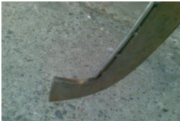
Figure 26: Detail of an injector knife with pipe.
