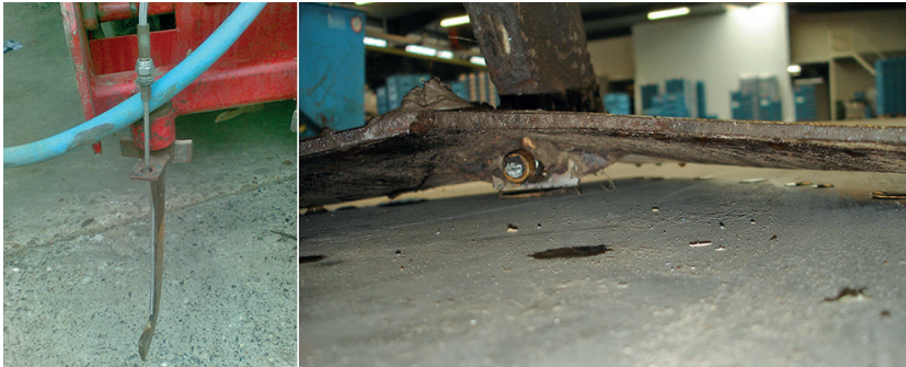
Figure 4: Left coultter with injector tube and right ploughshare with nozzle.
