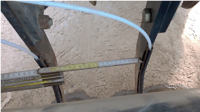
Figure 25: Measuring distance between the different injectors.
