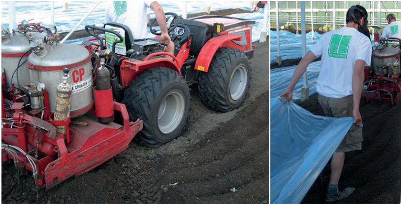
Figure 2: Injecting the disinfectant and manual plastic covering.
