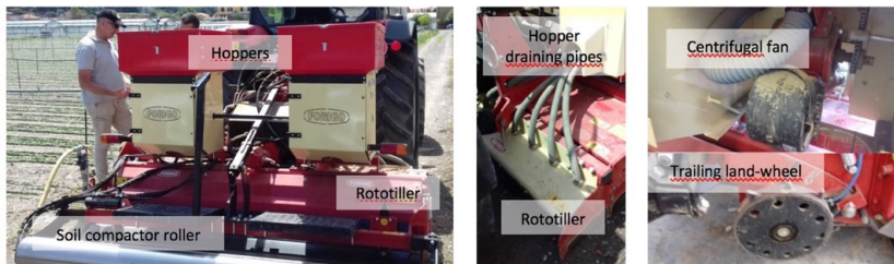
Fig. 2 - Example of solid fumigant applicator combined with a soil rototiller (Photo G. Oggero)
