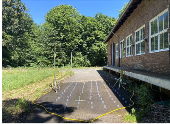
Fig. 2. Calibrating procedure for spatial uniformity testing needed for CU coefficient. Own study.
