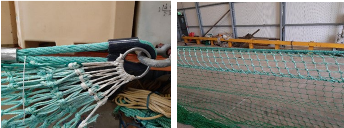
Fig 2.3.4 Steel ring of mounted upper wing tip alongside the eye of the headline after mechanical pulling of the wing (left panel). Some initial distortion in the wing meshes that should equalize after some use.
