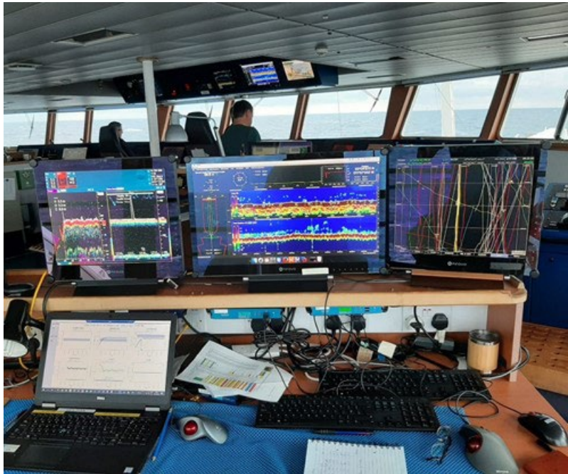
Fig 3.1.3 Aft bench on Celtic Explorer where scientists monitor survey and trawl parameters on a Scanmar bridge unit (top left monitor), MARPORT unit (top middle monitor) and location in proximity to historic commercial and survey data on a Sodena Chart Plotter (top right monitor). A custom application in R to plot and log median values in real-time for the local database thus DATRAS, is running on the laptop.
