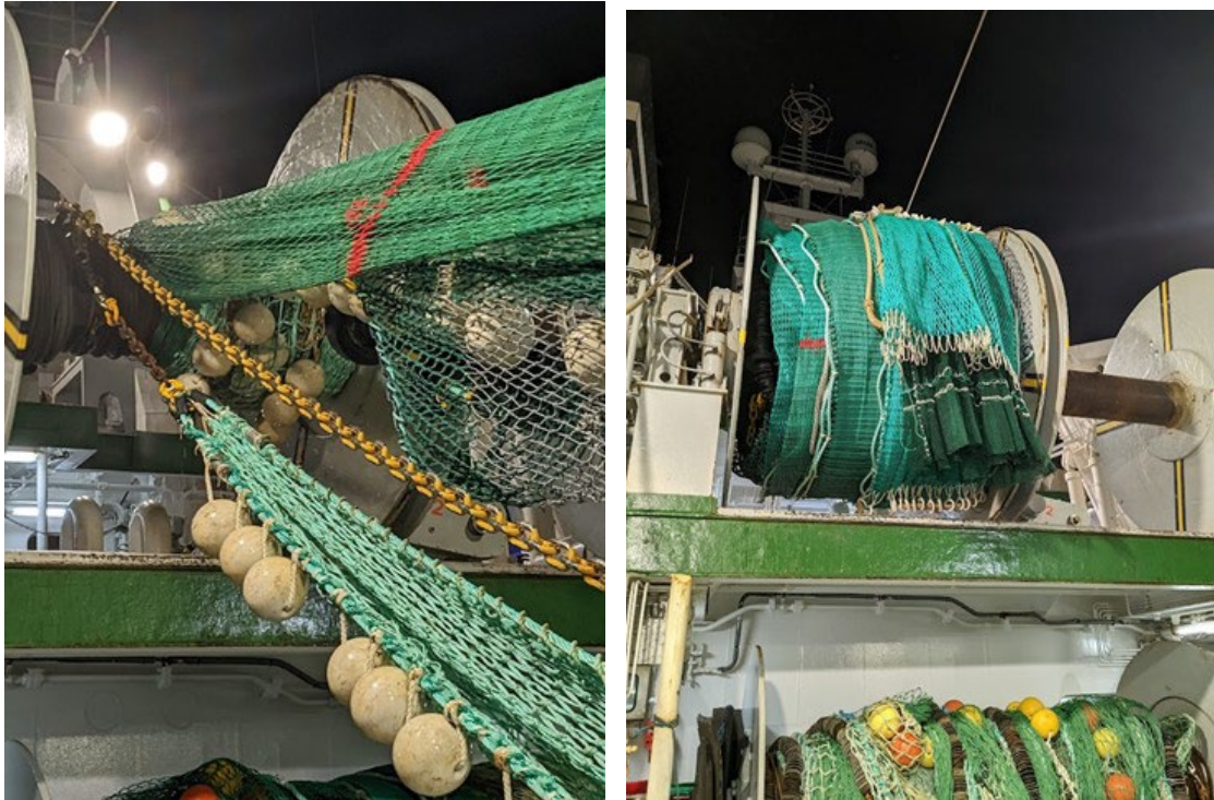
Fig 4.1 Showing the lower chain legs and floatation of the BT237_A being hauled onto the upper net drum on the Celtic Explorer (left panel). Fully stowed away the volume of net (excluding net drum core) was 7.25 m 3 and c.1,713Kg.
