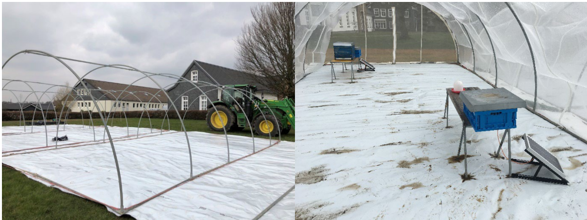
Figure 1 Setup of the ‘robbers tests’ in 2021. Left: covering the floor with plastic tarpaulins, which enabled counting of bees on the tent floor. Right: Setting up a test with one hive and one food source (the photo has been taken before the hive has been moved into the tent).
