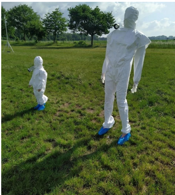
Fig. 1 Mannequins (adult/child) used for experiments dressed with coverall, gloves and plastic shoe covers
