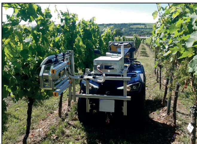
Fig. 1: The new phenotyping platform PHENOquad (left) with the PHENOboxx (right), a multi sensor setup used for data acquisition in grapevine breeding research. 1) Multi spectral camera (400-1.000 nm) 2) VNIR LED light Bars 3) TOF camera 4) GPS system 5) Ambient Light Sensor (ALS).
