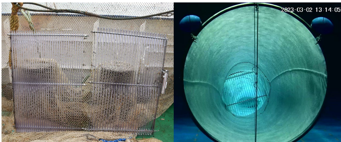
Figure 5.1: Plastic grids as bycatch reduction device. Left: Plastic grids with different bar spacing as tested in April 2023; Right: Test of plastic grid in flume tank.
