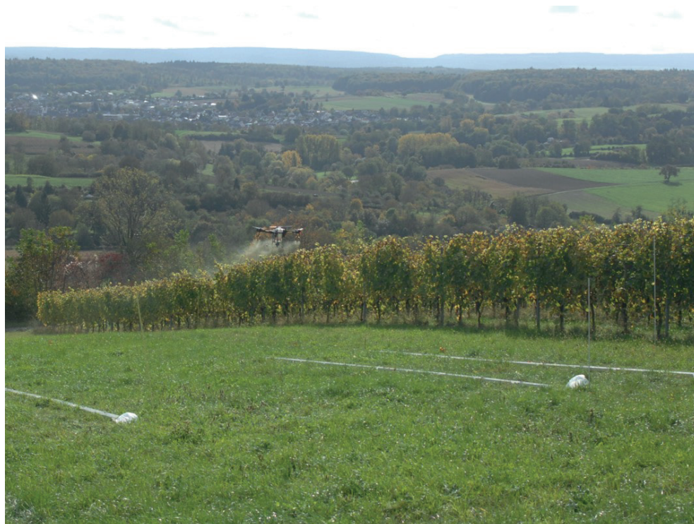
Fig. 3. View on the inclined vineyard in Weingarten during a test with the drone applying the test liquid, the short grass canopy on the downwind area and the planks supporting the petri dishes for drift sediment collection
