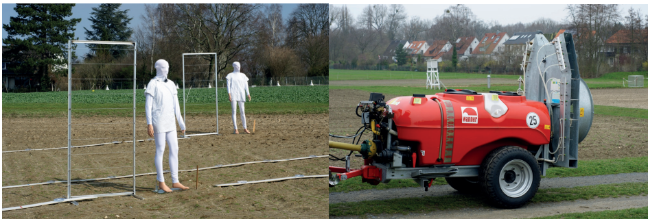
Fig. 3. Test setup for the first field trials following JKI Guideline 7-1.5 for drift measurements.
