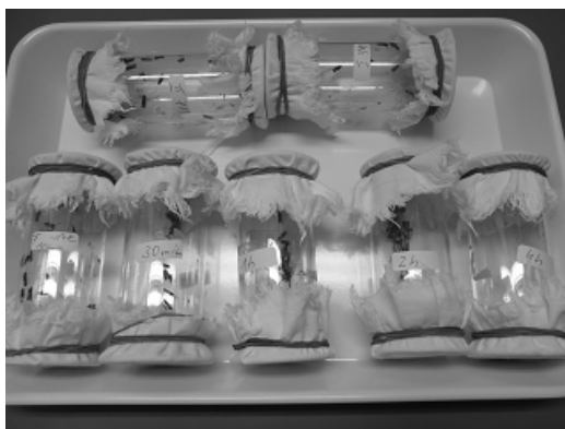
Figure 1 Glass tubes for exposure of adult moths after treatment with -14^\circ\text{C} .
