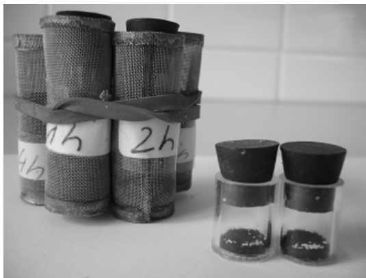
Figure 2 Small glass tubes for exposure of drugstore beetle eggs, and egg cages enclosed into wire mesh cages for testing.
