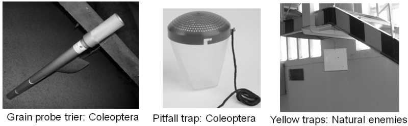
Figure 1 Devices used for sampling: grain trier, pitfall trap and yellow sticky trap.
