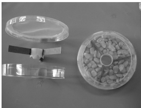
Figure 1 Multiple choice device for testing suspensions; a - lid with screening, b – central ring and cardboard tabs; c - base of the Petri dish; d - Petri dish with maize grain.
