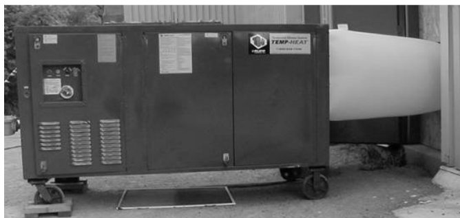
Figure 1 Propane-fired heater (Temp-Air) heater (source of heat for studies in Figure 3 and 4). The door was sealed with plywood, and a flexible fabric duct delivered heated air through a hole cut in the plywood,
