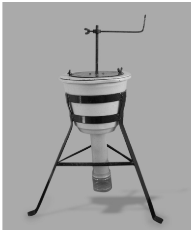
Figure 1 Outer view of pulse beetle egg removal device .
