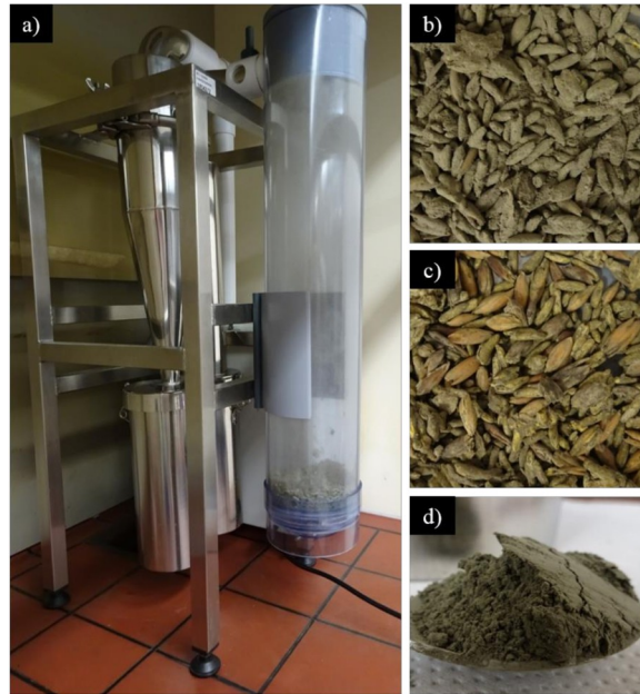
Fig 2. Mycoharvester® System. Mycoharvester® equipment, version 5b (a); substrate colonized by Metarhizium anisopliae before (b) and after harvest (c); pure conidia of Metarhizium anisopliae (d).
