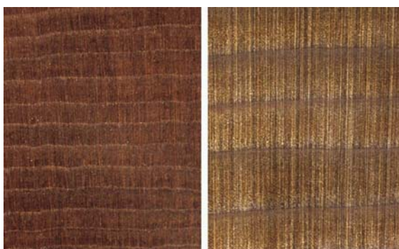
Figure 7: Alerce = Fitzroya cupressoides (CITES Annex I, left) and Western Red Cedar = Thuja plicata are virtually indistinguishable given their similar structure. The aromatic odour and yellowish hue of Western Red Cedar, however, is of much help in separating the two timbers
