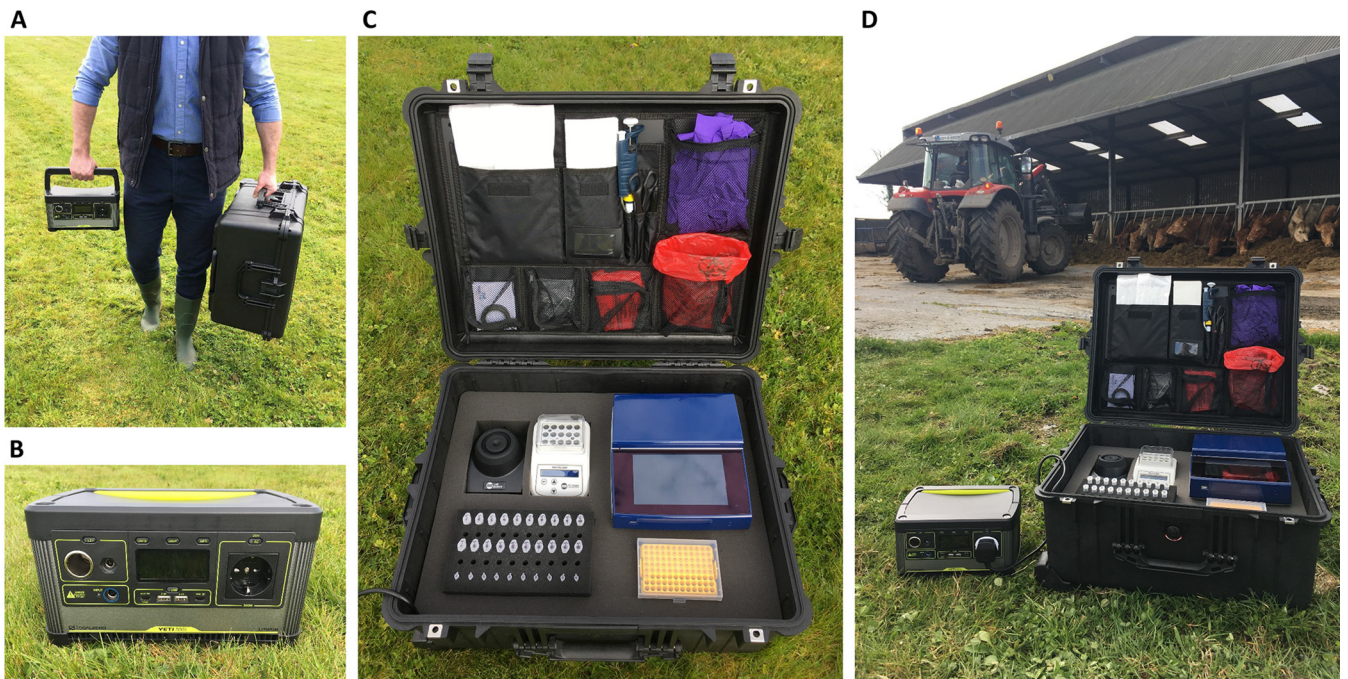
FIG 2 Portable diagnostics workstation. (A) Manual workstation transport. (B) Goal Zero power source. (C) Mobile workstation containing thermostatic fluorometer, mini dry bath, vortex, protector case, laboratory accessories and reagents for DNA extractions and LEC-LAMP reactions. (D) On-site application.
