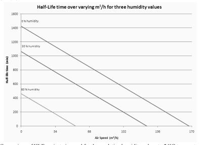
Figure 3 Comparison of HLT against air speed for three relative humidity value at  $\sim$ 24°C temperature.
