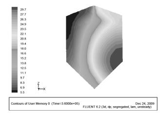
Figure 2 The distribution of phosphine concentration (mg/L) on a diametrical plane in a circular silo containing cotton seed after 100 hours of operation. The phosphine is introduced into the silo through a small hole on the lower right of the plane whence it disperses non-uniformly through the grain, the effect of which is exacerbated by the sorption on and reaction by of the fumigant on the grain.
