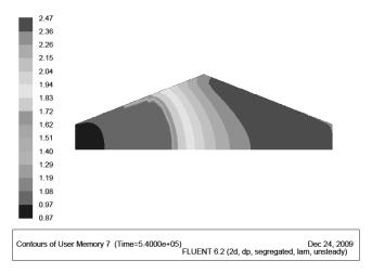
Figure 1 The ratio of potential population increase of *Rhyzopertha dominica* in wheat that has an initial moisture content of 12% (wet basis) and temperature of 35°C, after having been aerated for 150 hours with air that has a temperature of 10°C and a humidity of 0.007 kg water/kg dry air. The specific flow rate of the air is 2 litres per second per tonne of grain.
