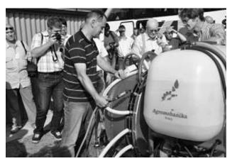
Fig. 4 Determination of the nozzle output of a vineyard sprayer at Hodonin
