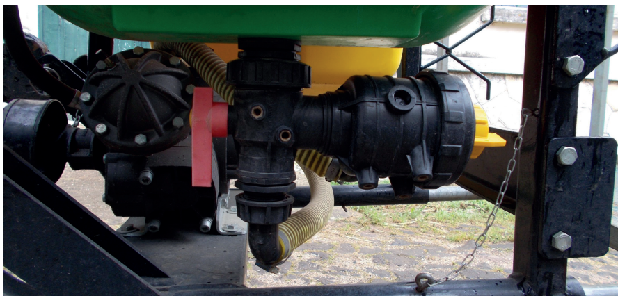
Figure 10. Isolated device allows to dismount the filter even with full tank
