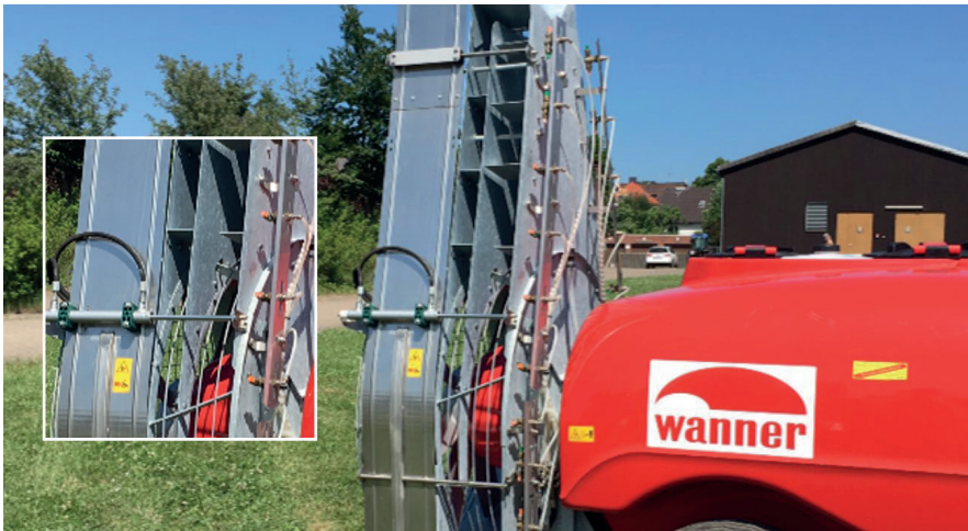
Figure 12. Device for individual side control of air assistance in orchard sprayers. By closing the outer side drift can be reduced
