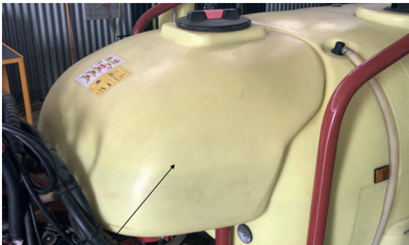
Figure 16. A rinse water tank for cleaning purposes is mandatory for all boom and orchard sprayers (except for orchard sprayers with a main tank of 400 l or lower).
