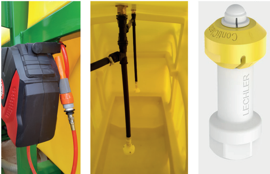
Figure 17. Special tool for external cleaning of the sprayer (left); device for automatic internal cleaning of the sprayer's tank (centre); special nozzle for internal cleaning of the tank (right).
