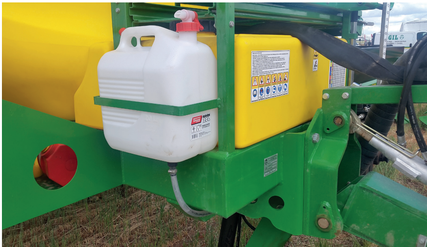
Figure 18. Clean water tank (minimum 15 l) shall be installed in the sprayers for safety purposes.
