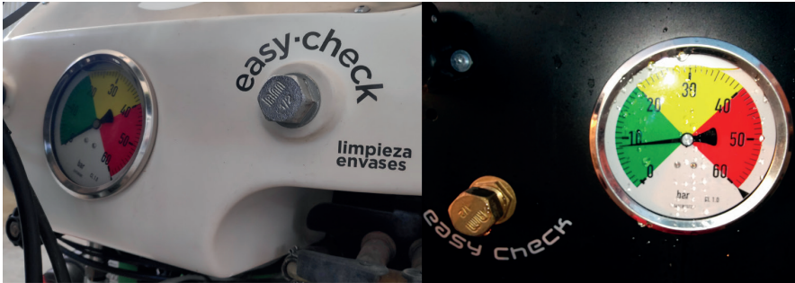
Figure 14. The sprayer shall be provided with a device for an easily connection of instruments used during the mandatory inspection of sprayers in use according ISO 16122. Left: easy adaptor for pump tester; right, easy plugging adaptor for testing manometer.
