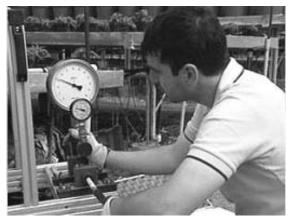
Fig. 3 Pressure gauge tester
