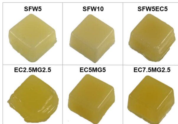
Figure 1. Photographs of oleogels based on rapeseed oil and different concentrations and/or combinations of sunflower wax (SFW), ethyl cellulose (EC), and monoacylglycerides (MG).
