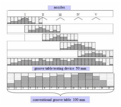
Fig. 4. Method of converting volumes of liquid table testing device (grooves 50 mm) for the table conventional patternator (grooves 100 mm)- virtual boom sprayer.Results of first tests and conclusion
