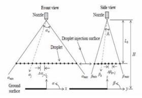
Fig. 1. Schematic showing the virtual nozzle with spray cloud boundaries, droplet injection surface, and droplet injection positions: x,y and z, coordinates;  $\alpha$  and  $\beta$  angular coordinates defining the spray boundary and droplet positions; H, nozzle height above the ground, Lb liquid sheet break-up length. [SIDAHMED and al., 2005].
