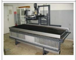
Fig. 3. Device to complex measurements of agricultural nozzles
