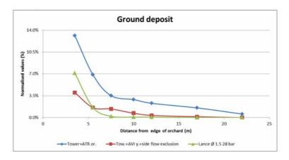
Fig. 3. Normalised values of ground deposit retrieved for each of the tested equipment (average values from three replicates).
