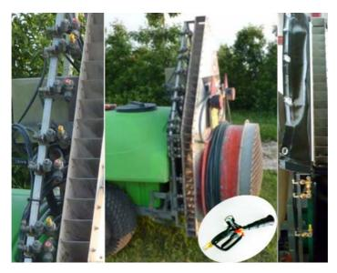
Fig. 15. Equipments compared during the test: particular of the side flow exclusion device (right), the double crown of nozzles (left) activated indipendently and the handheld gun fitted with manometer (oval box).
