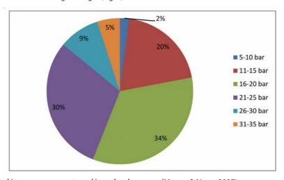
Fig. 5. Working pressures most used in orchard sprayers (MARTINS & NUNES, 2007).
