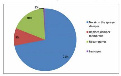
Fig. 11. Most common defects in pumps (Martins & Nunes, 2007).
