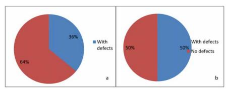
Fig. 9. Defects in pressure gauges of field crop sprayers (Martins & Nunes, 2007a), defects in pressure gauges of orchard sprayers (Martins & Nunes, 2007b).
