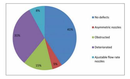
Fig. 10. Most common defects in nozzles (Martins & Nunes, 2007).
