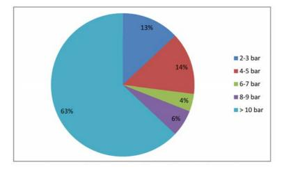
Fig. 6. Working pressures most used in boom sprayers (Martins & Nunes, 2007).
