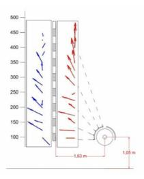
Fig. 8. Projection of air velocity vectors on a single vertical plane passing through the measure points.
