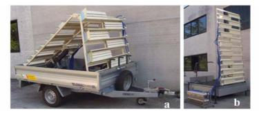
Fig. 2. The droplets intercepting patternator: a. folded on the bottom of the trailer; b. placed vertically.
