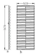
Fig. 14. The droplets intercepting patternator: a.lateral view; b. front view (dimension in mm).
