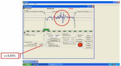
Graph 1. Cross distribution of IDKT 120-04C nozzles in use. Tested on Herbst scanner patternator SPRAYERTEST 1000
