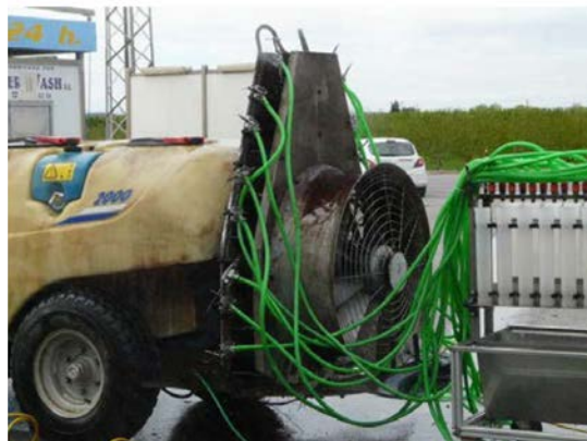
Fig. 1. Nozzle flow rate measurement in an air assisted sprayer.
