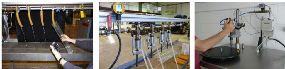
Fig. 2. Three methods for nozzle airflow measurement, graduated cylinder and stopwatch (left), air-tight nozzle adaptor (centre) and nozzle flow rate bench (right).
