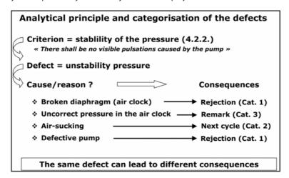
Fig. 3. Analytical principle and categorisation of the defects.
