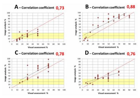
Fig. 3. Correlations between visual assessment and image analysis measurements of coverage on WSP samples obtained by teams A, B, C and D during the field experiment verifying the calibration effects. Preferable coverage range is between 10 and 30%.
