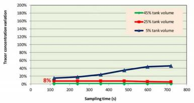
Fig. 16. Glass microspheres concentration in samples taken out of the 200 l lacking of any agitation system.
