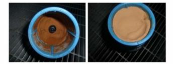
Fig. 11. Example of filters obstructed with nutshell powder.
