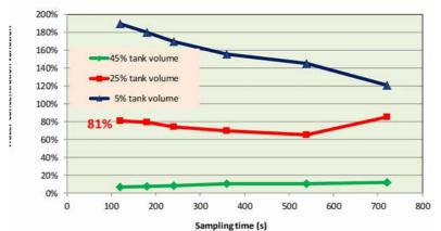
Fig. 14. Glass microspheres concentration in samples taken out of the 200 I tank when the agitation system was activated.
