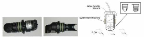
Fig. 1. Flow meters "Wolf" model manufactured by Arag company and example of a paddlewheel sensor.
