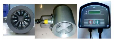
Fig. 4. Second type of sensor instrument equipped with an axial fan flow meter in a cylindrical body.
