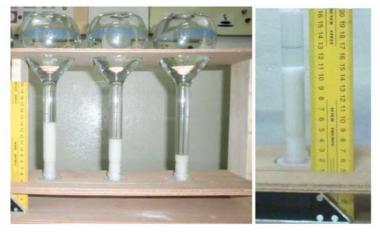
Fig. 8. Graduated flasks containing the tracer suspensions upturned and positioned in supports provided with a graduated scale to read the amount of sediment deposited in the flask neck.
