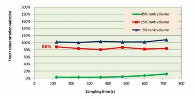
Fig. 12. Glass microspheres concentration in samples taken out of the 600 I tank when the agitation system was activated.
