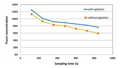
Fig. 9. Comparison between tracer concentrations measured in the tank samples after different sampling times, with and without the agitation system activated (600 l tank capacity).
