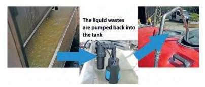
Fig. 6. Example of system for collection and properly disposal of all wastes produced during sprayer inspection/calibration.
