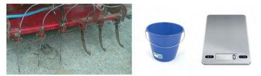
Fig. 4. Soil-disinfection machine injectors, pattern measurement.
