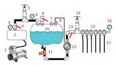
Fig. 3. Hydraulic scheme of a soil-disinfection machine.
