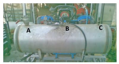
Fig. 6. Pesticide tank with unsafe filling valve (A), safe depressurising valve (B) and safety valve (C).
