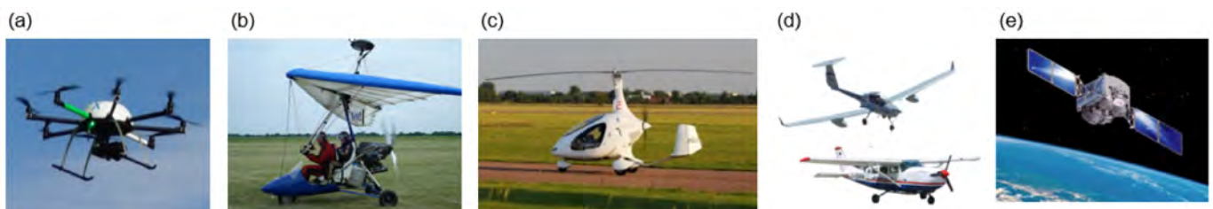
Figure 4. Different air- and spaceborne remote-sensing platforms for assessing geomorphodiversity, geomorphic traits, their changes and disturbances: (a) unmanned aerial vehicles (UAV or drone), (b) microlight—gravity-controlled; (c) gyrocopter or microlight helicopter; ((d)—top) ECO-Dimona; ((d)—bottom) Cessna and (e) satellite (from Lausch et al. [47]).
