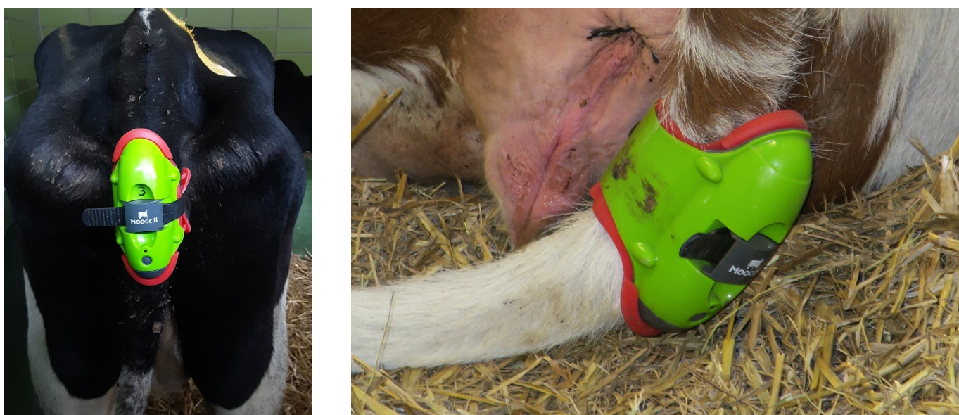
Figure 1. The Mocoall® (Mocoall Ltd., Dublin, Ireland) remote calving sensor attached to the tail of late pregnant cows.
