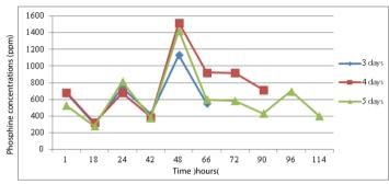
**Fig. 1** Average phosphine concentrations inside the maize stacks during fumigation at the different times with ECO<sub>2</sub>FUME<sup>\*</sup> dosage 25 g/m<sup>3</sup> (350 ppm).
