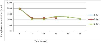
**Fig. 3** Average phosphine concentrations inside the maize stacks during fumigation at the different times with  $ECO_2FUME^*$  dosage 70 q/m<sup>3</sup> (1,000 ppm).
