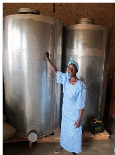
Figure 3. Airtight metal can capacities larger than 1.8 MT “become hard to operate” (George, 2011). Image: FAO 2015.
