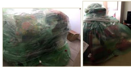
Picture 2: Well shrunk fumigation cube (left), and badly placed shrink tape (right).
