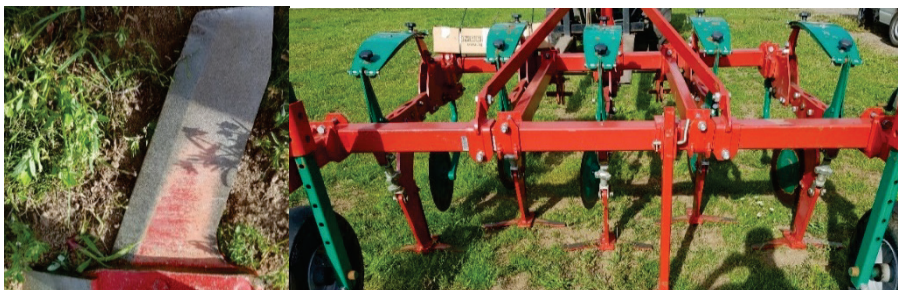
Figure 1 The “Kverneland horizontal root cutter” is a tractor pulled 5 sheered tillage machine. Each sheer has a diameter of 50cm and can run up to 30cm deep into the soil, cutting and fragmenting root and shoot parts in the process.
