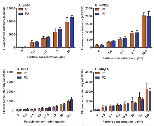
Figure 7. Intralaboratory comparison, conducted with the revised SOP, of DCFH<sub>2</sub> oxidation by (A) SIN-1, (B) NPCB, (C) CuO, and (D)  $Mn_2O_3$ , and expressed as arbitrary fluorescence units. The data represents those of two contributing partners operating from the same facility, and is presented as the mean and SD of at least three independent replicates.
