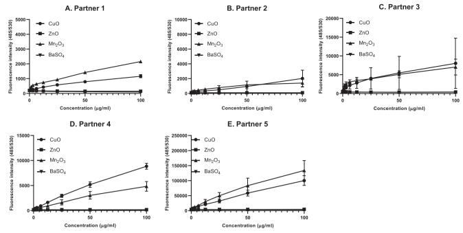
Figure 1. (A–E) Interlaboratory comparison by five partners of DCFH<sub>2</sub> oxidation by ZnO, BaSO4,  $Mn_2O_3$ , and CuO using provisional SOP (conducted during first interlaboratory comparison). Data represents the mean and SD of at least three independent replicates, and are expressed as arbitrary fluorescence units.
