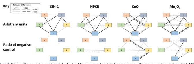
Figure 3. Pairwise differences between partners during first interlaboratory comparison study. In each column are differences shown in evaluation of SIN-1, NPCB, CuO, or  $Mn_2O_3$ , and rows are differences found when using arbitrary fluorescence units or when data was normalized to negative control values; statistically significant differences between mean values are shown with lines, and between slopes with dotted lines.
