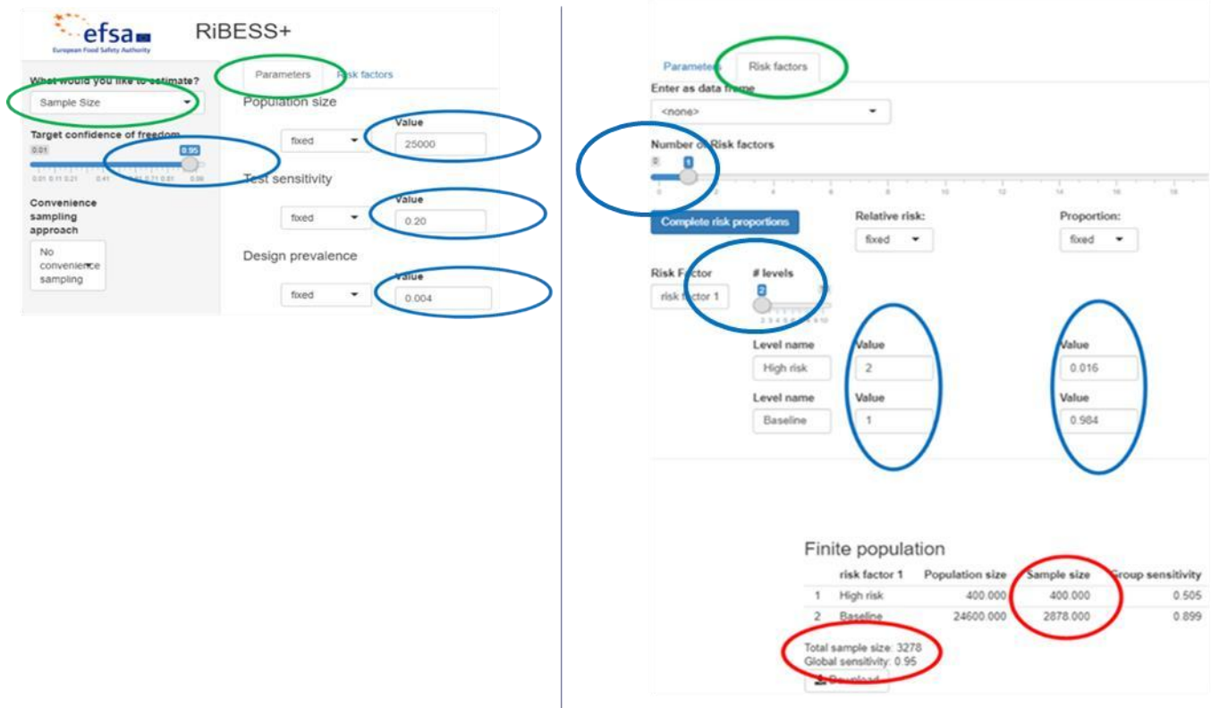
Figure C3: Screenshots of RiBESS+ for calculating the number of hectares to inspect with integration of the risk factor to achieve an overall 95% confidence level and a 0.4% design prevalence given 20% method sensitivity (20% confidence level at the hectare level) (the green circles are the chosen functionalities, the blue circles are the input values of the survey parameters, the red circles are the estimated output values)
